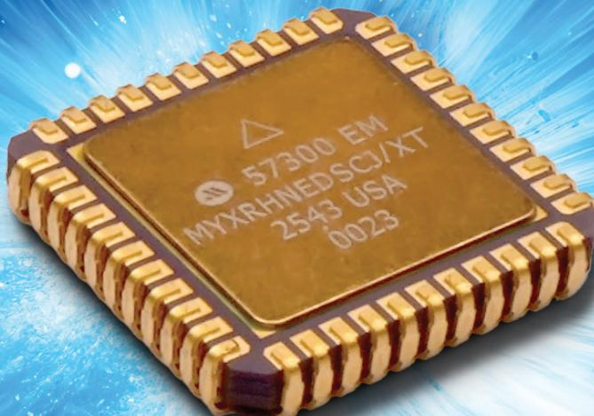
The Standard-Performance Nuclear Event Detectors (NED) features a 2X increase in radiation dose rate sensitivity, and 50%+ reduced response times at 10X lower overdrive levels relative to legacy devices. With integrated differential drivers providing SWaP reduction, improved noise immunity & reduced delay times.
